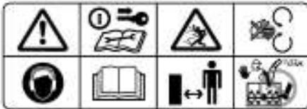
1. Remove the ignition key before any operations.
